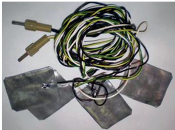
Figure 1. Galvanic cell and lead electrodes for galvanization procedures
