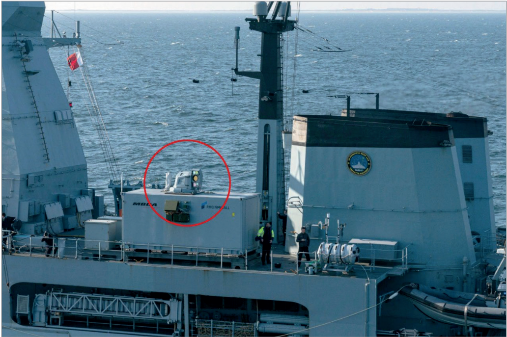
Figure 4. German anti-UAV laser system LWD 33
