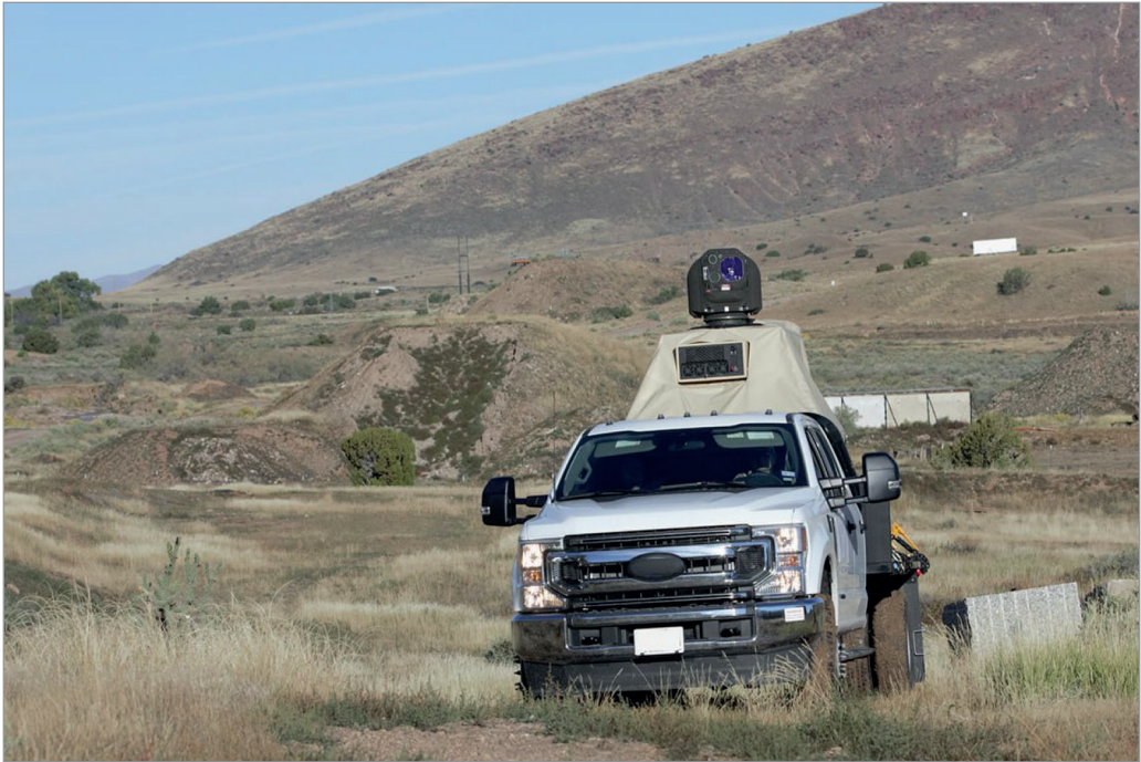
Figure 2. British anti-UAV laser system Raytheon HELWS 28
